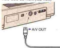
Using the NEO GEO RGB cable (FCG-9), connect the console's A/V output terminal to the television's 21-pin input terminal.
