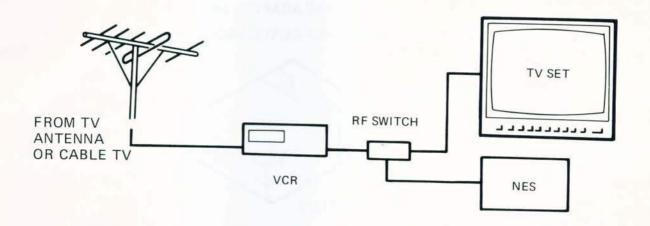
IF THERE IS A CABLE CONNECTED BETWEEN THE VCR AND THE UHF TERMINAL ON THE BACK OF YOUR TV SET, LEAVE THAT CABLE AS IS.
