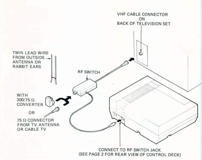
NOTE: If a VCR is already connected between the antenna and the VHF terminals on the back of your TV set, the RF switch must be installed between the VCR and the TV as shown below:
