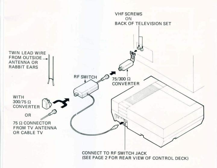
(ii) If your TV has a VHF cable connector, connect the RF switch and NES as shown below.
