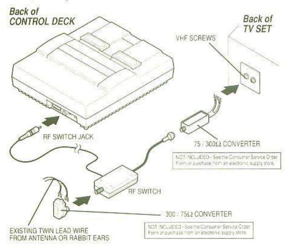
NOTE: This method of connection will produce mono sound only (the left and right stereo channels are mixed).
