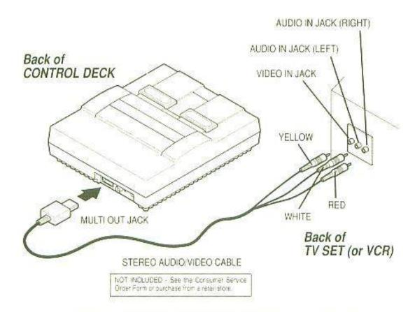
NOTE: This is the only method of connecting the Super NES Control Deck to a TV to get the full effects of the stereo sound. It is also possible to connect the audio output of the Control Deck to a stereo system. For additional information on this type of connection call: 1-800-255-3700
