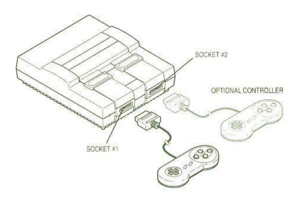
All Super NES Controllers are identical and can be plugged into either socket number, but the *select* and *start* buttons will work only on the controller plugged into socket #1. For one-player games or when you are playing a game alone, the controller must be plugged into socket #1.
