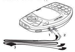
The headset lead functions as the antenna of the radio, so let it hang freely.
